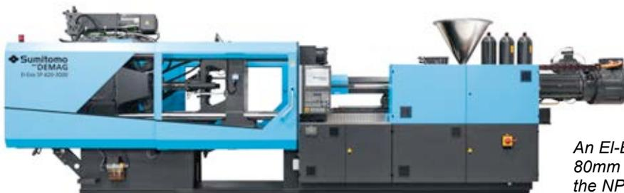
*An EI-Exis SP 420/820-3000 with 80mm barrier screw will be featured in the NPE demonstration.*
