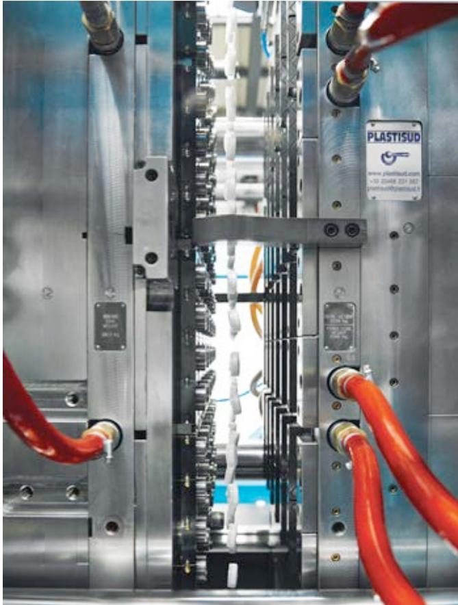
*A new generation of high-speed molds combines advanced cooling design with Plastisud hot-runner technology specially engineered for high throughput.*
