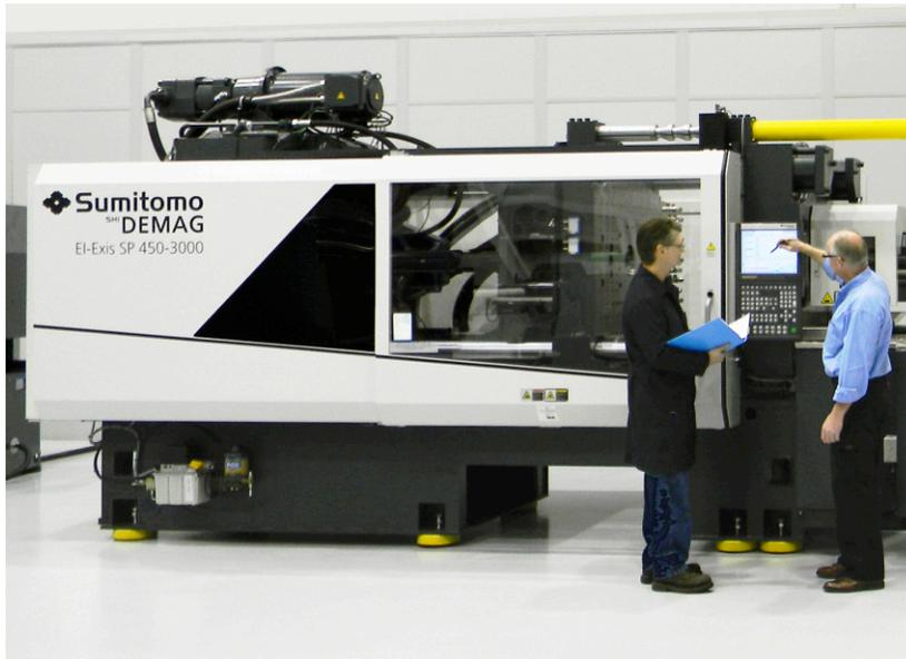
*Sumitomo (SHI) Demag Project Engineer, Robert Budowanec, and Field Service Engineer, Sean Mulholland, discuss the NC5 plus control capabilities of the EI-Exis SP 450 hybrid in the new Technology Center. This machine will be running an ultra-high-speed, multi-cavity closure molding application at the opening of the facility.*
