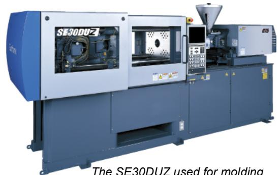
*The SE30DUZ used for molding the DNA sample collection tubes is equipped with an optional 16 mm SL Screw Assembly.*
