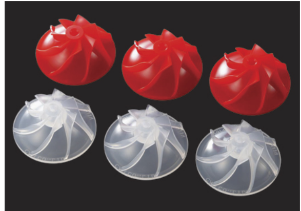
The demo featured a 3-cavity, cold runner mold for the 1.9-gram parts.
