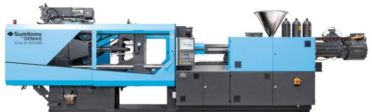
An EL-EXIS SP 450/920-3000 (500 U.S. tons) is molding 1- gram HDPE water bottle caps on a 2.3-second cycle in a 96-cavity SCHÖTTLI AG (NPE Booth 49000) hot-runner mold.
