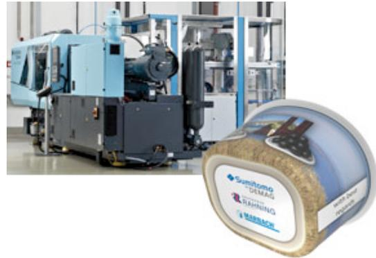
The Marbach-developed process uses a "full cover label placer" that inserts the banner and base label in a single stroke. Previous IML solutions required a partition on the container base that meant that full coverage with the label in the injection mold was not possible.
