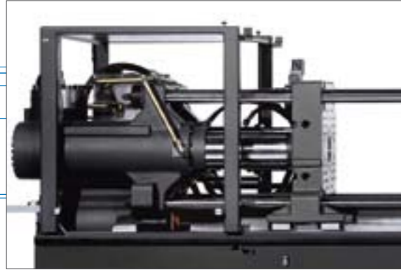
Fig. 1: Fully hydraulic clamping unit
