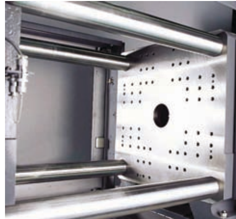
The increased width between tie bars on the SE-DUZ allows installation of large mold bases and increases the work space for mold setup.
