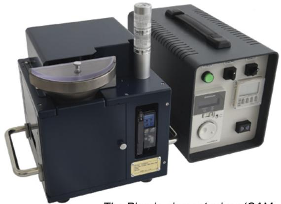
*The Pigmic pigment mixer (CAM Co., Ltd.) precisely weighs and meters colorant to the screw.*
